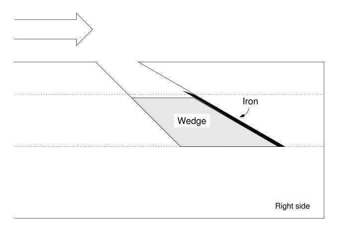
Once the iron and wedge are suitably set, affix the plane to your bench. You can do this by clamping it in a vise, or by attaching a clamp to the plane and then clamping the clamp to your bench. It's also possible to use the plane simply by pushing the front of the plane up against a stop projecting above your benchtop.
